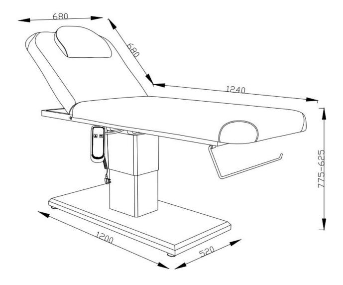
Seat height: 775-625mm/ Total Height(backrest 90 degree): 1660-1305mm Seat width: 680mm/ Seat depth: 1240mm
